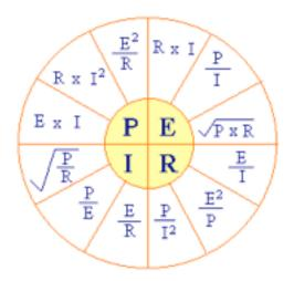
Ohm's law can be applied to an entire circuit, or to any portion of it. This may be stated:
